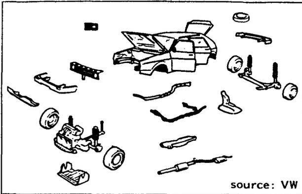
Fig. 13 Modular design of an automobile
