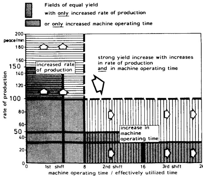
Fig. 7 Increased yield by increased rate of production and/or machine operation time
