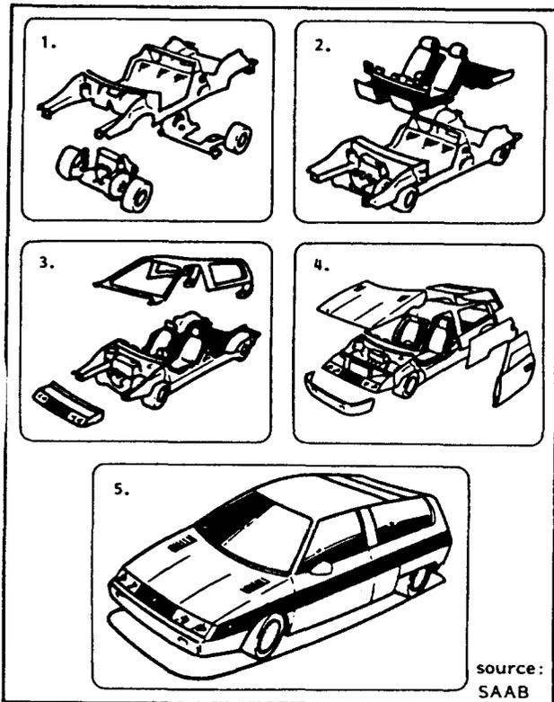
Fig. 14 Module concept for a final car assembly
