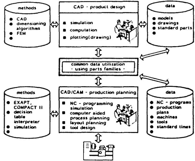
Fig. 5 Integrated system for product design and production planning
